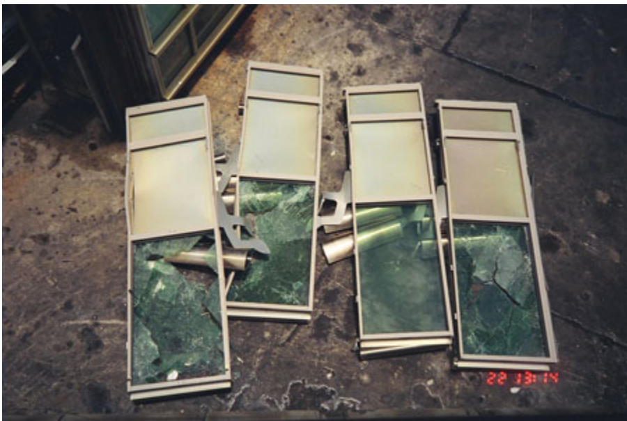
During onsite tests, unitized curtain wall frames failed when exposed to negative loads.
