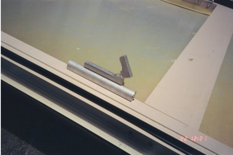
Deformed anchor hook – analysis would reveal that hook was manufactured using an incorrect alloy.
